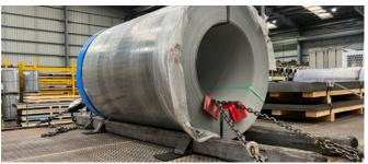
Rubber load mat can be used for repeated use between steel loads and steel decks to increase friction and eliminate the extremely slippery steel on steel surfaces.
