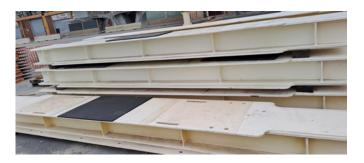
Rubber load mat can be used for a variety of steel and concrete construction materials transport and storage to prevent slippage or damage to finished items.
