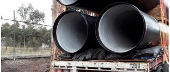
Rubber Load Mat can be used for load restraint during transport of complex items such as pipes and can be bonded to support parts & bolsters.
