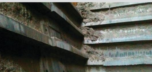
Reglin wear liners installed on screen underflow chute walls.
